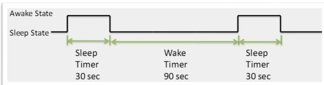
The above diagram shows the transitions between the Sleep state and Awake state based on the sleep and wake timers.
